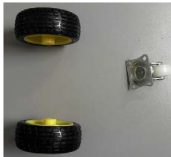
Figure 6.3 – Two wheels with a castor
