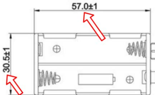
Figure 6.16 – A battery box product drawing with dimensions
