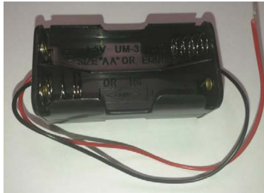
Figure 6.14 – The 4 x AA battery box we use with the motors
