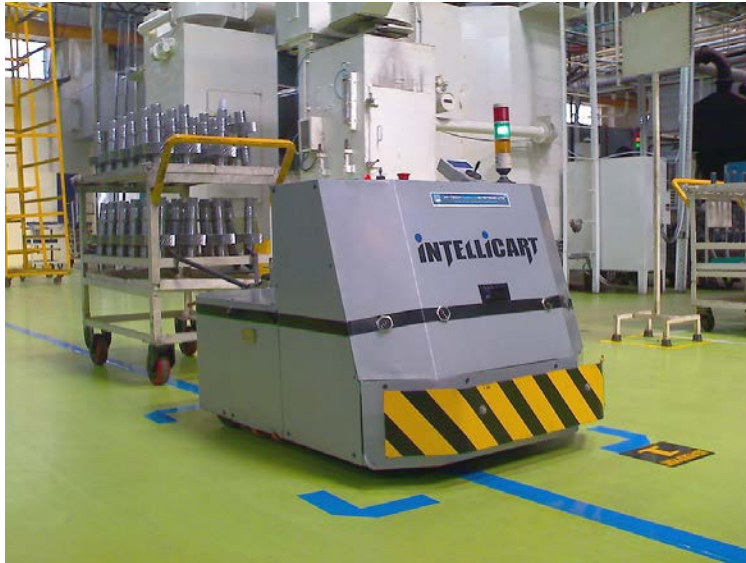
Figure 14.1 – IntellCart – a line-following industrial robot by Mukeshhrs [Public domain]
