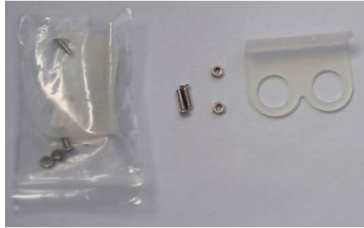
Figure 8.8 – Ultrasonic HC-SR04 sensor brackets with the screws and hardware
