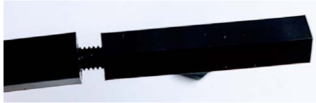
Figure 12.6 – Joining the standoff posts
