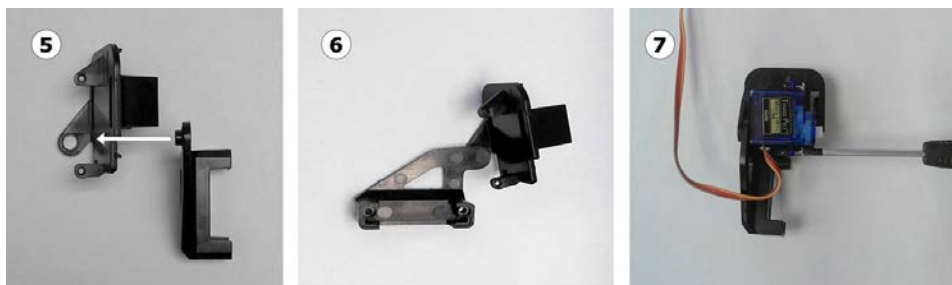
Figure 10.12 – Assembling the left arm and tilt plate
