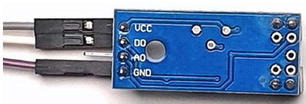
Figure 11.7 – The sensors with cable connections
