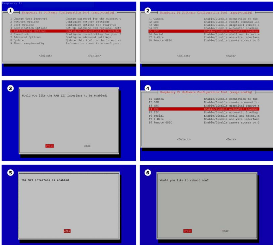
Figure 7.1 – Using raspi-config to enable SPI and I2C
