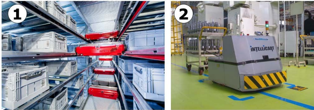
Figure 1.8 – Warehouse robot systems: Stingray system by TGWmechanics [CC BY-SA 3.0 ( https://creativecommons.org/licenses/by-sa/3.0/ )], and Intellicart by Mukeshhrs [public domain]
